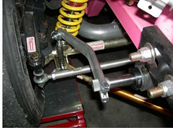
7. Place the car on the ground at proper ride height and adjust the placement of the mounting blocks in the clamps to ensure the turnbuckles are as close to vertical as possible. They should not lean forward/backward, or right/left. When everything is set correctly, slide the arms back off the swaybar.
