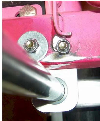
You may find you need to grind or cut some oil cooler bracket mounting out of the way on the inner side of the frame as shown above.
