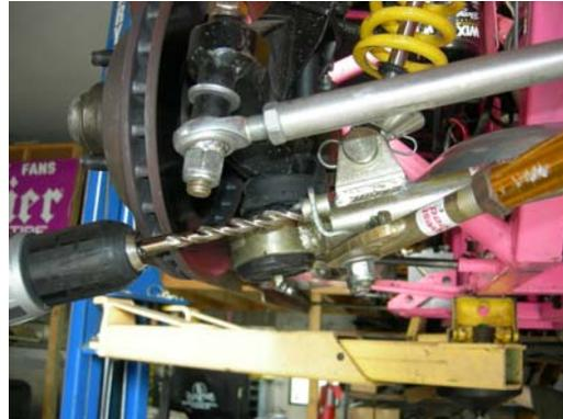
3. Place both mounting blocks for the swaybar under the front of each side of the framerail as shown. Measure approx. 3" back from the front end of the framerail and clamp the mounting block at this point. Slide the swaybar through the white nylon bushings in the mounting blocks until it is centered in the frame. If the chassis has been twisted, you may need to have one block farther back on the frame than the other to ensure the bar is not "binding" in the nylon bushings.
