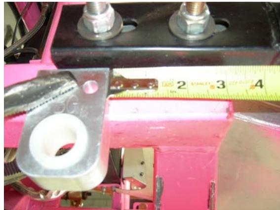
4. Slide a 7/8" clamp from the outside of each end of the swaybar and clamp up against the edge of the white nylon bushing to keep the swaybar from sliding left or right in the mounting blocks.
